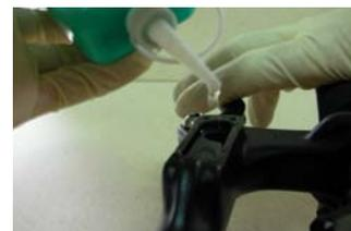
When you open the reservoir tank cover and find the fluid have been added or adding the fluid could not improve the brake power. You have to bleed the new fluid for banishing the added fluid and air form the hydraulic system.
