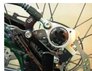
Always check the brake fluid in the reservoir tank, when you feel the brake is not enough brake power or no pressure point after confirming that hydraulic system of the brake is no leak.
