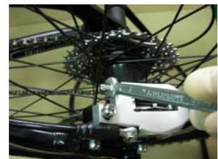
6. Connect the syringe and the caliper bleed screw. Gently push the syringe plunger with your thumb and squeeze the lever.
