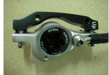
2. Mount the adapter to the fork or frame using fitting bolts(M6x1.0/18 mm) for Allen key 5 and keep “up” upward. Torque the bolts to 12.4Nm (110 in-lbs) For post mount forks, you need longer (M6x1.0/22 mm)bolts for installation. For that fork, torque the fitting bolts to 9.0 ± 0.55 Nm (80± 5 in-lbs)
