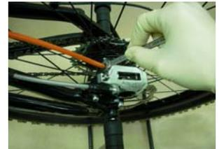
**Caution: Do not troque over! It will damage the opening of the caliper.**
