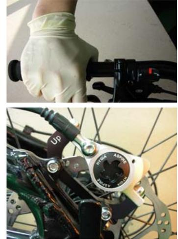
As you try to rotate the wheel to test the brake, do not worry the slight friction between the rotor and the pads. A slight drag noise is natural during the pads run in period. The drag will disappear gradually after using.
