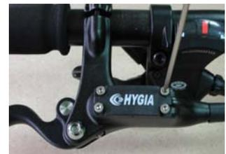
10. Install the original reservoir cover and squeeze the lever several times. Check the brake power again. Then, adjust the master cylinder body to optimum angle.
